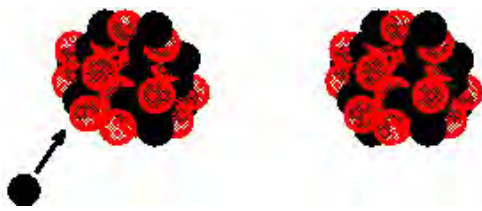
Figure 3. Before collision of neutron (black) with chlorine-35 nucleus, 17 protons (red) and 18 neutrons. After collision, neutron is captured, resulting in chlorine-36 with 17 protons and 19 neutrons.
