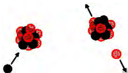
Figure 2. Before collision of neutron (black) with nitrogen-14 nucleus, 7 protons (red) and 7 neutrons. After collision, neutron is captured and proton is ejected, resulting in carbon-14 with 6 protons and 8 neutrons.
