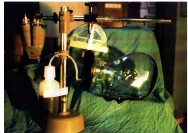
Figure 5. Specially modeled head for fluid flow simulation.
