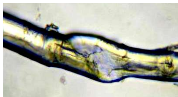
Figure 3. Microscope image of a single linen fiber colored with ArF laser. The mechanical damage in the middle shows a colorless inner medulla. Contrast-enhanced detail of figure 8 in Ref. [24]. Small shreds of the yellowed pcw are visible.
