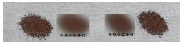
Figure 13. Same as figure 11, after four months. The stains have been blurred (middle section) in order to measure the average RGB values at the center of the blurred stains. © Niels Svensson.
