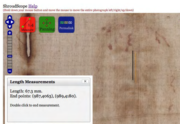
Figure 4. A length measurement was done along the nose on the Durante photograph. The measure icon has a redish hue: the ShroudScope is in measurement mode and no longer in panning mode. The black line shows the location of the measurement and the small popup window on the left shows the length as 67.3 mm (millimeter) and the two end-points of the yellow line as coordinates (987,4063) and (989,4180).
